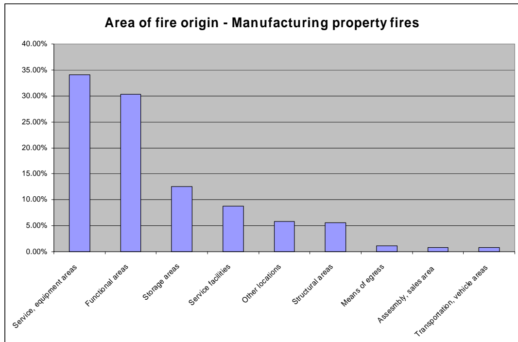
Figure 24 – Manufacturing: Area of fire origin
